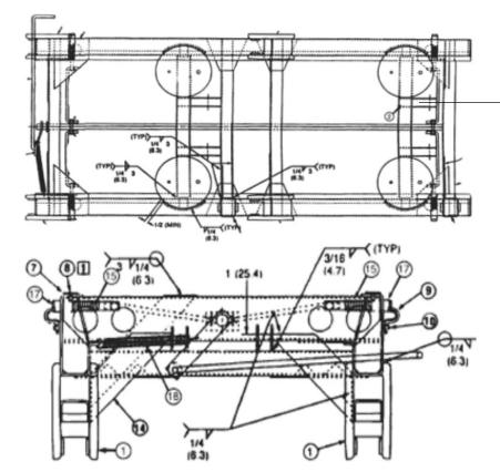
Part No. 20538-48 Slider Box - 48-3/8" frame width.
